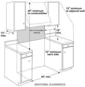
Allow 12" minimum clearance to an adjacent wall on each side.
