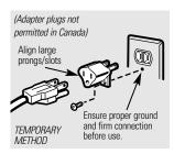
The larger slot in the adapter must be aligned with the larger slot in the wall receptacle to provide proper polarity in the connection of the power cord.
