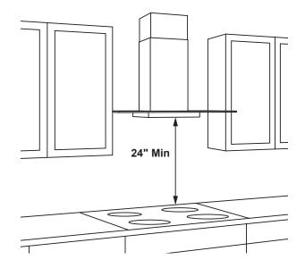
The vent hood must be installed 24" min. above the cooking surface. For optimal performance, installing the hood more than 36" above the cooking surface is not recommended. The hood installation height above the cooking surface depends upon ceiling height. The telescopic duct cover conceals the ductwork running from the top of the hood to the ceiling.
