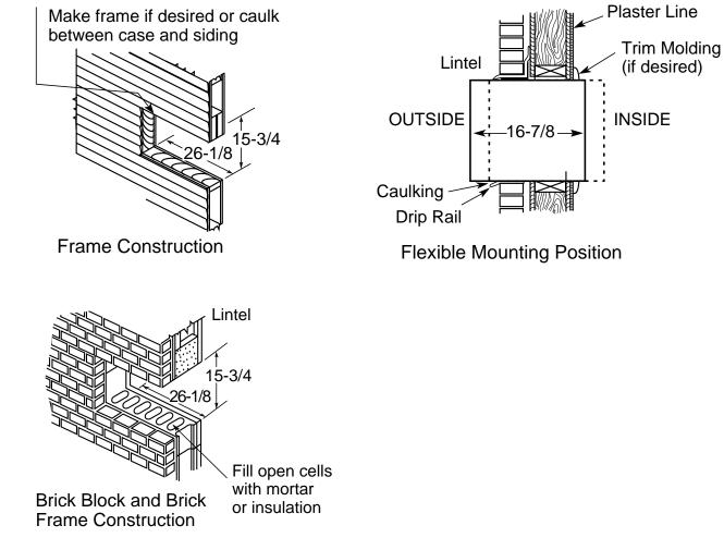
**Installation Information:** A finished opening of 26-1/8" x 15-3/4" clear of intrusions is required. Keep clearance of 4" from side walls. Brick veneer or frame walls should have wood studding surrounding case to provide firm anchoring with screws. Case can be fastened directly to brick or block walls with screws sunk in lead expansion shields.
