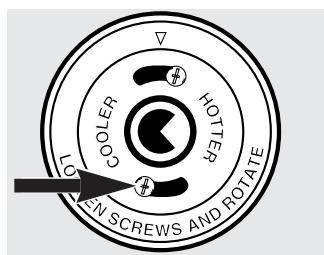
The lower screw moves toward COOLER to decrease the temperature.
