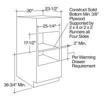
Additional clearances between the cutouts may be required. Check to be sure the oven supports above the warming drawer do not obstruct the required interior depth and height. See warming drawer installation instructions for details.
