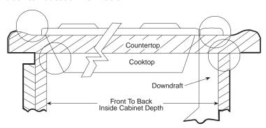
Note: Pay special attention to the four areas of potential interference circled at left. 2" of FLAT countertop is needed behind rear edge of cooktop to accommodate downdraft vent cover. (Required to maintain U.L. or AGA approvals.) It is recommended that gas and/or electrical service for cooktop and downdraft should be in adjacent cabinet to right.
