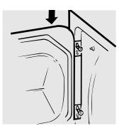
**3** Rotate the door 180°. Insert it on the opposite side of the opening by moving the door *IN* and *DOWN* until the top hinge and the bottom hinge are resting on the top screws inserted in step 1.
