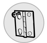
2 Loosen top screw from each hinge on the dryer face half way. With one hand holding the top of the door and the other hand holding the bottom, remove the door from the dryer by lifting it **UP** and **OUT**.
