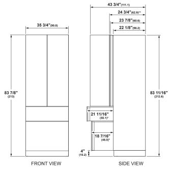
\*Depth dimension without handle. Statement handle adds 2 9/16" depth. Minimalist handle adds 2 1/8" depth. \*\*Includes 3/4" door panel
