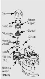
IMPORTANT: Be sure small holes in the gasket are centered directly over the small holes in the nozzle and venturi housing.
