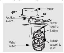
If you don't get a reading in the display, with faucet open, pull the sensor from the valve outlet port. Pass a small magnet back and forth in front of the sensor. You should get a reading in the display. If you get a reading, shut off water supply, unhook the in and out plumbing and check the turbine for binding.
