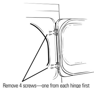
Remove 4 screws—one from each hinge first
