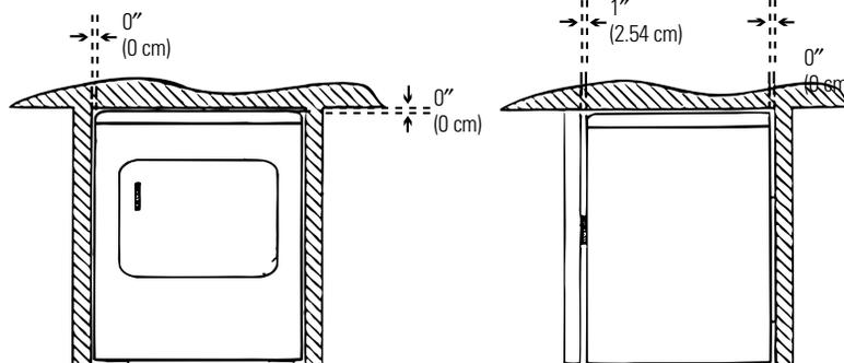
**NOTE:** Undercounter and stack models—0" (0 cm) for sides, rear and top
