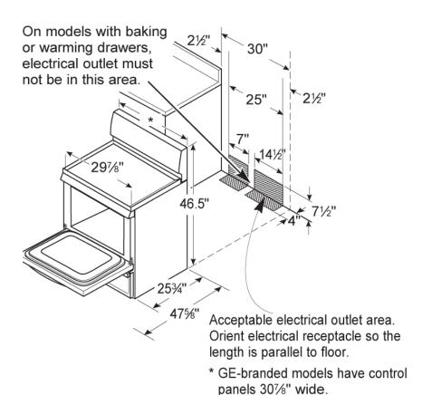
**NOTE:** Use a 4' power cord to prevent interference with the storage drawer. Power cords  $4\frac{1}{2}$ ' to 6' long may have to be dressed to allow for proper drawer closing.
