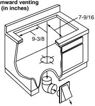
Note: In some cabinets, the sides may need to be scooped or cut down 2" as shown and the corner braces removed in order to accommodate the cooktop.
