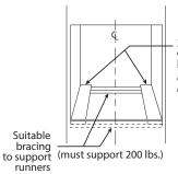
2 x 4 or equivalent runners level with bottom of cutout and flush with sides of cutout or solid bottom floor.
