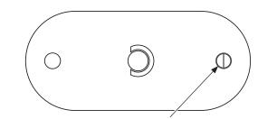
Right adjustment screw for extra-large burner
