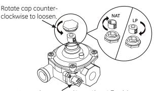
Lever shown open (Oven Shut Off only) PUSH LEVER DOWN TO CLOSE
