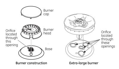
B. Using a 7 mm or 9/32" nut driver, remove the top burner orifices. These may be accessed through the burner opening in the base.
