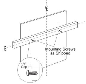
Adjust depth of supplied mounting screws in the wood support until they protrude 1/4" forward. This 1/4" gap will provide clearance to hang the hood. **IMPORTANT:** Framing must be capable of supporting up to 150 lbs.
