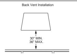
In this installation, the ductwork running from the back of the hood goes directly into the wall.
