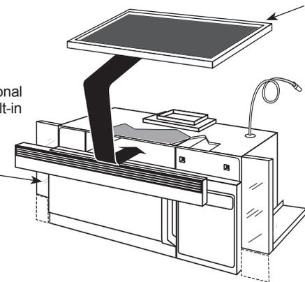
Filter Kit JX81J—Recirculating Charcoal Filter Kit To be used when the Spacemaker microwave oven cannot be vented to the outside.
