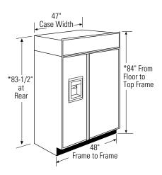
\* Shipping height. The refrigerator can be adjusted to fit into a cutout that is 83-1/2" min. to 84-1/2" max. height Note that the top case trim at the front is 1/2" higher and will overlap upper cabinetry or soffit. Use leveling legs and wheels for height adjustment.
