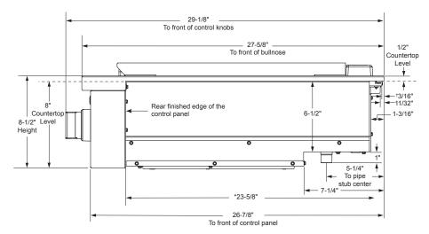
\* Minimum cabinet cutout depth from the back of the rear trim to the back finished edge of the control panel typically, the minimum cabinet depth (front to back). Maximum cabinet cutout depth is 26" minus the countertop overhang.
