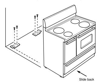
**5.** Slide the range into place making sure the rear legs are trapped by the ends of the brackets. The range may need to be shifted slightly to one side as it is being pushed back to allow the rear legs to align with the brackets. Remove the storage drawer to inspect brackets or grasp the top rear edge of the range and carefully attempt to tilt it forward to make sure the range is properly anchored.
