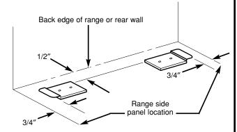
Brackets attach to the floor at the back of the range to hold both rear leg levelers. When fastening to the floor, be sure that screws do not penetrate electrical wiring or plumbing. The screws provided will work in either wood or concrete.
