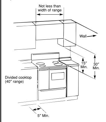
**NOTE:** There is a minimum 5" clearance required from the left side of the range to a wall. This clearance is needed to open the left side oven door or to remove the left oven shelf.
