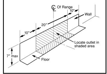
The figure below shows the recommended installation relationship of the ranges to the vertical walls of the surrounding structure. Please note the following:
