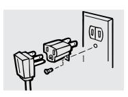
This is a temporary method. UL-listed adapters are available at most hardware stores. Because most 2-prong outlets are not grounded, we strongly advise against using an adapter plug. However, a temporary connection may be made where local codes permit and if the 2-prong wall outlet is properly grounded.
