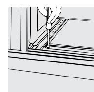
*3* Assemble the 2 leveling bolts and nuts to the support brackets.
