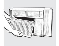
The air filter is behind the front grille insert and should be checked and cleaned at least every 30 days or more often if necessary.
