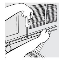
5 On the outside, turn the leveling bolts until each one makes contact with the wall. Make sure the back of the case tilts 1/4" to 3/8" lower than the front. Tighten the nuts.
