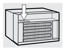
*Write down the model and serial numbers here.* They are on a label on the left side of the air conditioner below the air discharge area. Staple your receipt to the inside back cover of this manual. You will need it to obtain service under warranty.
