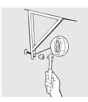
4 Attach the support brackets to the bottom of the case with 1/2" screws, 2 on each side.
