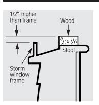
A storm window frame will not allow the air conditioner to tilt towards the outside and will keep it from draining properly. To adjust for this, attach a piece of wood to the stool.
