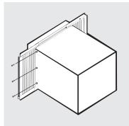
3 Peel the backing off the bottom window gasket and place onto the backside of the window stool.
