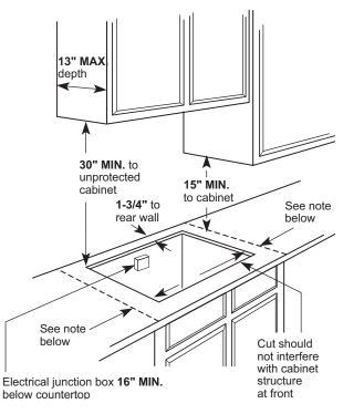
**NOTE:** This cooktop has been approved for 0" spacing to adjacent surfaces above the cooktop. However, a 6" minimum spacing to surfaces less than 15" above the cooktop is recommended to reduce the exposure to steam, grease spatter and heat.
