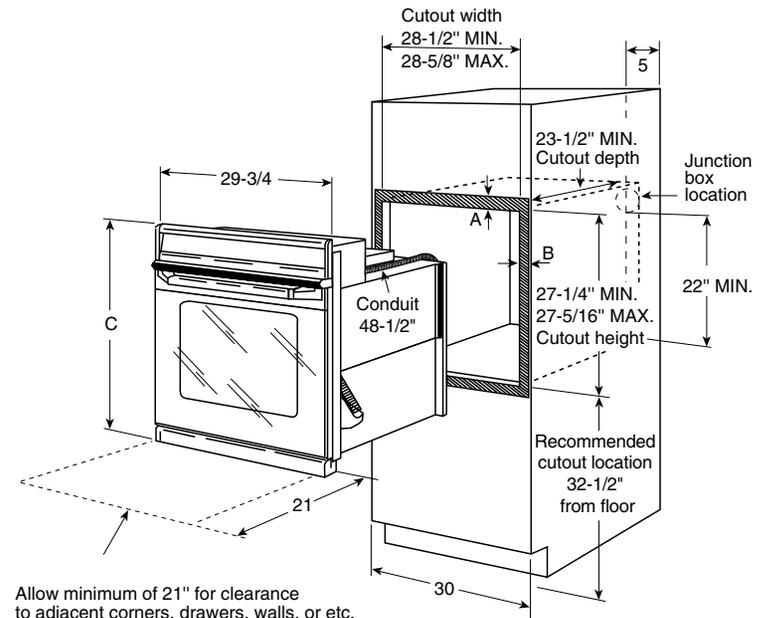
Allow minimum of 21" for clearance to adjacent corners, drawers, walls, or etc.
