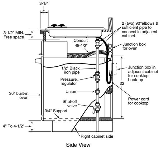
This installation is to achieve minimum gap between bottom of countertop and control panel.
