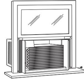
C Reinstall the control to the panel housing by replacing the 2 screws you removed earlier.
