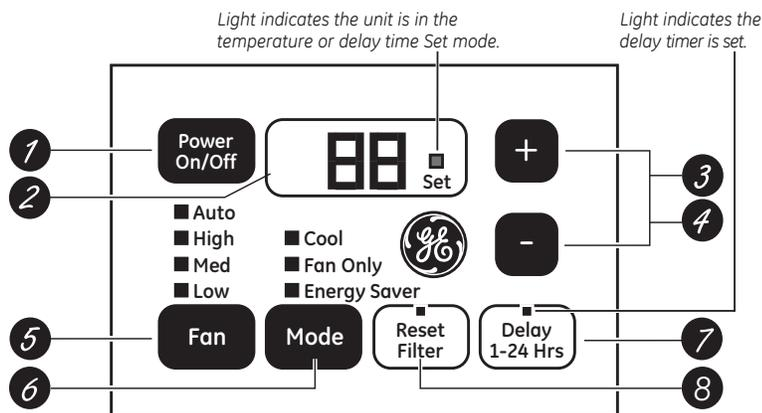
NOTE: The display always shows the room temperature except when setting the Set temperature or the Delay timer.
