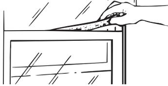
**NOTE:** If the gasket supplied does not fit your window, obtain appropriate material locally to provide a proper installation seal.
