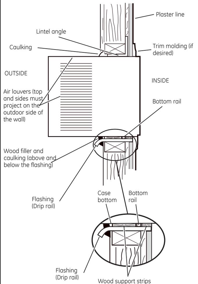
**B** Place the air conditioner into the case. For specific instruction, refer to the Window Installation Instructions.
