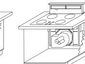
**Note:** Telescopic downdraft vents are not recommended to be installed with cooktops that are flush mounted.
