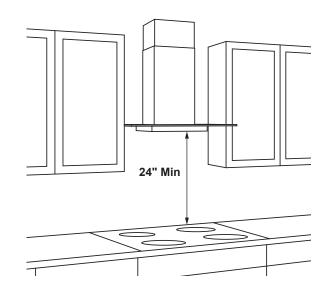
The vent hood must be installed 24" min. above the cooking surface. For optimal performance, installing the hood more than 36" above the cooking surface is not recommended. The hood installation height above the cooking surface depends upon ceiling height. The telescopic duct cover conceals the ductwork running from the top of the hood to the ceiling.
