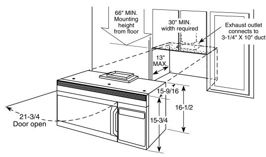
**Important Information:** When installing the microwave oven over a range, allow minimum of 2" from bottom of Counter Saver Plus microwave oven to top of range backguard to allow for removal of light covers.
