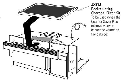
**Ventilation Options:** The microwave oven is designed for adaptation for the following three types of ventilation:
