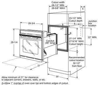
A=Allow 1" overlap of oven over top and bottom edges of cutout. B=Allow 11/16"-3/4" for overlap of oven over side edges of cutout.
