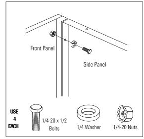
• Stand the assembly up and bolt the front panel to the side panels with bolts, washers and nuts as shown. (2 on each side).
