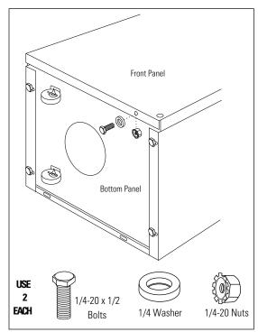
• Place the front panel on the assembly. Install bolt with washer from the bottom into the base and secure with nuts. Do not tighten.
