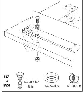
• Install front brace to base with 4 bolts and washers through the top and secure with nuts on the bottom. Do not tighten.
