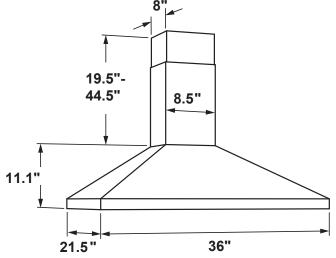
The vent hood must be installed 24" min. above the cooking surface. For optimal performance, installing the hood more than 36" above the cooking surface is not recommended. The hood installation height above the cooking surface depends upon the ceiling height. The telescopic duct cover conceals the ductwork running from the top of the hood to the ceiling.
