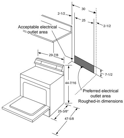
\*Dimension from wall to front of closed oven door handle is 27-3/8".
