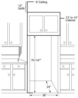
\*The rough-in dimension of 70-1/4" is minimum and is measured from the finished floor to top of opening (or the underside of the overhead cabinets). For Models with Trim Kit: If trameless style cabinets are planned for above the refrigerator, you may need to consider adding a maximum of 1/4" (70-1/2") to height of opening to allow additional clearance between cabinet doors and top of refrigerator trim when cabinet doors are in open position.
