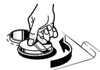
**NOTE:** To open detergent cup after it has been closed, simply turn the detergent cup handle counterclockwise until it releases. A snapping sound may be heard.
