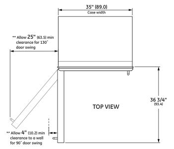
\*\*These units are equipped with a 2-position door stop. The factory set 130° door swing can be adjusted to 90° if clearance to adjacent cabinets or walls is restricted. Allow 15" minimum clearance to wall for pan removal. If the 90° door stop position is used, pan access is maintained but pan removal is restricted.
