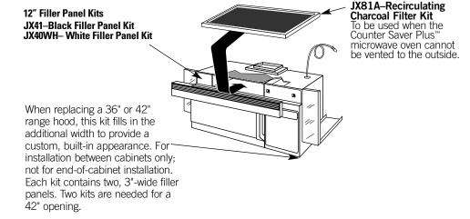
Ventilation Options: The Counter Saver Plus™ microwave oven is designed for adaptation for the following three types o ventilation: Outside Exhaust (Vertical–as shown above) Outside Exhaust (Horizontal) Recirculating Exhaust (Non-vented ductless–see Filter Kit Drawing)
