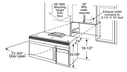
**Important Information:** When installing the Counter Saver Plus<sup>™</sup> microwave oven over a range, allow minimum of 2" from bottom of Counter Saver Plus<sup>™</sup> microwave oven to top of range backguard to allow for removal of light covers.
