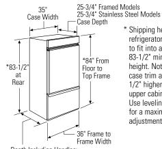
\* Shipping height. The refrigerator can be adjusted to fit into a cutout that is 83-1/2" min. to 84-1/2" max. height. Note that the top case trim at the front is 1/2" higher and will overlap upper cabinetry or soffit. Use leveling legs and wheels for a maximum 1" height adjustment.
