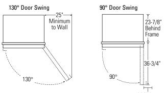
Allow 25" minimum clearance for a full 130° door swing. Allow 15" for pan removal. 4" Minimum to Wall
