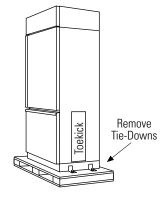
• Remove the four 7/16" bolts securing the straps to the skid.
