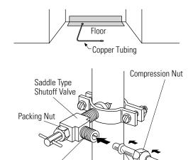
**NOTE:** It is best to install the valve into a vertical water pipe. If you install the valve into a horizontal water pipe, make the connection at the top or side to avoid drawing off any sediment from the water pipe.
