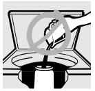
Do not pour anything into the agitator if the agitator cap or dispenser is removed.
