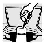
**The fabric softener dispenser** automatically releases liquid fabric softener at the proper time during the cycle.
