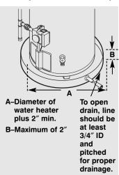
NOTE: The auxiliary catch pan installation MUST conform to local codes.
