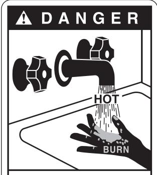
Water temperature over 125°F can cause severe burns instantly or death from scalds.
