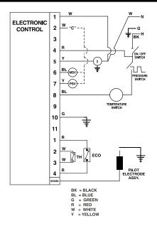
A CAUTION! Label all wires prior to disconnection when servicing controls. Wiring errors can cause improper and dangerous operation.
