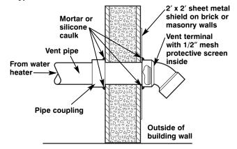
**HORIZONTAL VENT INSTALLATION**—Once the vent terminal location has been determined, make a hole through the exterior wall to accommodate the vent pipe. Vent pipe must exit exterior wall horizontally only. (See illustration.)
