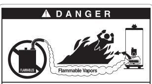
Vapors from flammable liquids will explode and catch fire causing death or severe burns,
