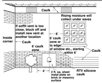
A WARNING: Moisture in the flue gas will condense as it leaves the vent terminal. In cold weather this condensate can freeze on the exterior wall, under the eaves and on surrounding objects. Some discoloration to the exterior of the building is to be expected. However, improper location or installation can result in severe damage to the structure or exterior finish of the building.
