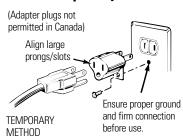
**CAUTION:** Attaching the adapter ground terminal to the wall receptacle cover screw does not ground the appliance unless the cover screw is metal, and not insulated, and the wall receptacle is grounded through the house wiring.
