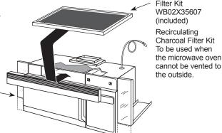
Filter Kit WB02X35607 (included) Recirculating Charcoal Filter Kit To be used when the microwave oven
