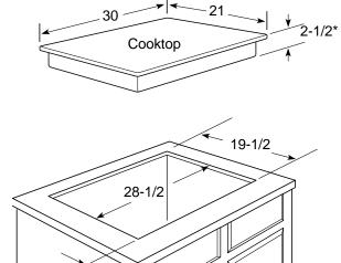
\*Depth of unit at conduit location (rear) is 4-3/4"
