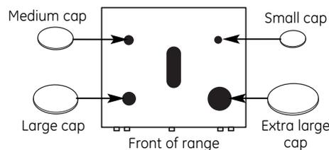
Make sure that the heads (on some models) and caps are replaced in the correct locations.
