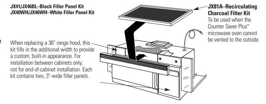
**Ventilation Options:** The Counter Saver Plus<sup>™</sup> microwave oven is designed for adaptation for the following three types of ventilation:
