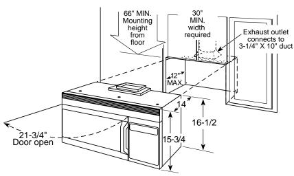
**Important Information:** When installing the Counter Saver Plus microwave oven over a range, allow minimum of 2" from bottom of Counter Saver Plus
