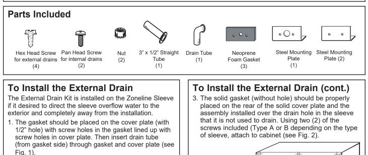
Enter screw through the back of mounting plate Fig. 1
