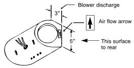
When the blower is in position, snap the blower retainer bar toward the front into the indent.
