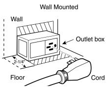
Recommended acceptable electrical outlet area. Orient the electrical receptacle so the length is parallel to the floor.
