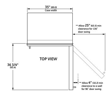
\*\*These units are equipped with a 2-position door stop. The factory set 130° door swing can be adjusted to 90° if clearance to adjacent cabinets or walls is restricted. Allow 15" minimum clearance to wall for pan removal. If the 90° door stop position is used, pan access is
