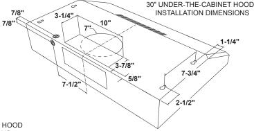
Exhaust outlet connects to  $3-1/4" \times 10"$  rectangular duct. Vent top or rear. Includes rectangular damper.
