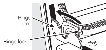
Push hinge locks up to lock.
