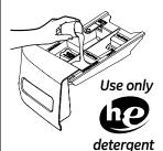
Open the dispenser and add detergent, bleach and fabric softener, as desired. This washer multi-doses the detergent in small amounts during wash to achieve the best cleaning.
