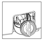
to drain from the filter. STEP 3: Turn pump filter counterclockwise and remove the filter slowly to let the water drain.
